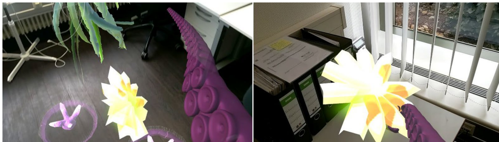
Fig. 4 Tentacle extending and retracting according to the myoelectric signals from the user to grasp a virtual game object
